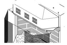
Figure 10 - Removing Screen
